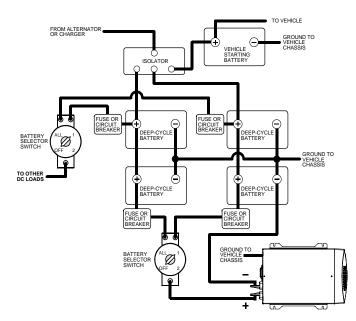
Figure 7 Configuration for Heavy Loads
