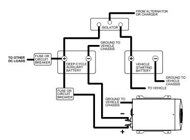
Figure 6 Configuration for Normal Loads
