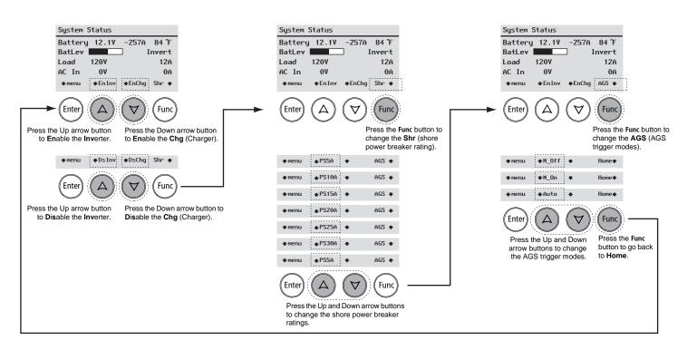
Figure 13 Freedom SW System Status Screen - Soft Key Navigation
