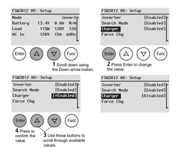
Figure 20 Selecting and Changing a Configurable Setting
