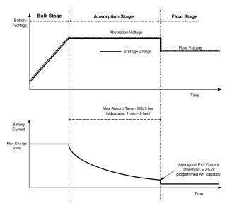
Figure 34 Three-Stage Battery Charging Cycle
