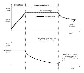
Figure 35 Two-Stage Charging Cycle
