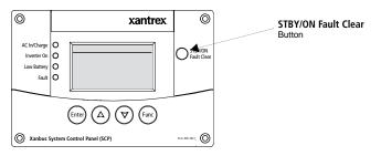
Figure 14 Xanbus SCP STBY/ON Fault Clear Button
