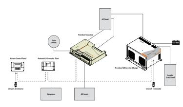
Figure 1 Typical Xanbus System Diagram
