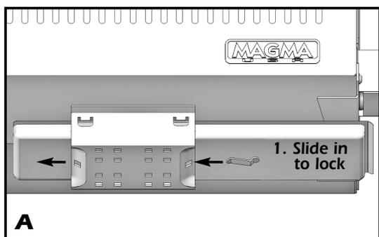
1. Slide Grease Tray into either side of the mounting bracket to lock.
