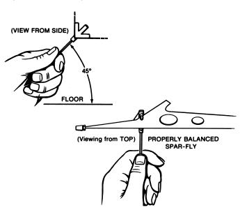
When balanced, tighten nut. Test sensitivity by walking past Spar-Fly in a closed area before mounting.
