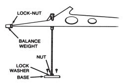
On wood spars, attach base to masthead using long brass wood screws.
