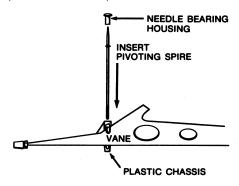
Do NOT attempt to insert from the bottom. Follow these instructions precisely. Now, with finger, press needle bearing housing into hole in top of plastic chassis. Continue to press housing against a solid object (such as a table) until it is seated, but don't press so hard that spire bearing becomes jammed. Test to make sure vane spins freely on spire. No lubrication is necessary.
