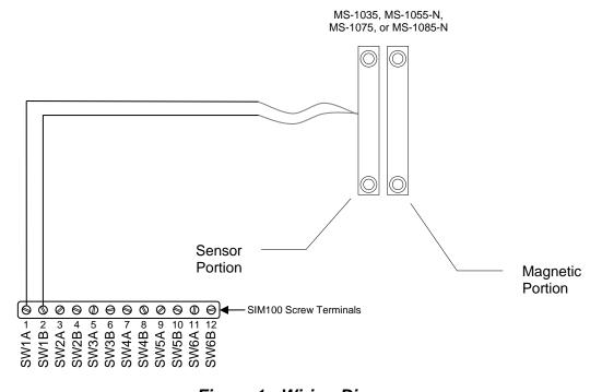
Figure 1 - Wiring Diagram
