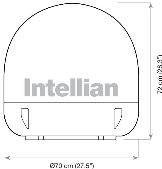
Figure 08: Radome Dimension of i6/i6P
