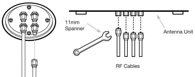
Figure 12 : Connectors on Bottom of Antenna
