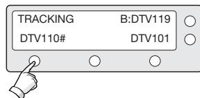
3. Press LEFT soft key for tracking Satellite C.
