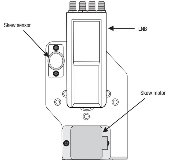
Figure 21 : Auto LNB Skew Angle Adjustment
