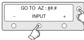
4. Input position value for azimuth (AZ) axis.
