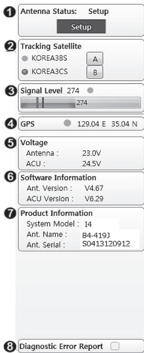
① **Antenna Status:** Displays the status of the current mode of the antenna.
