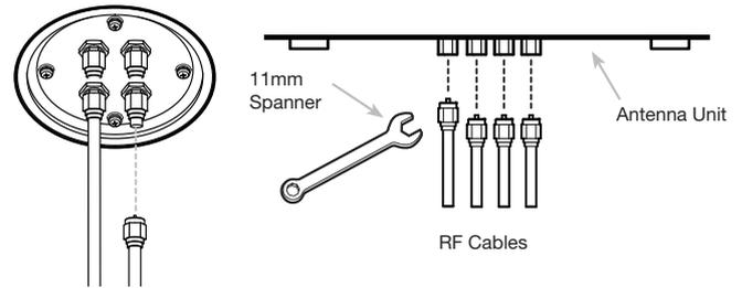
Figure 12 : Connectors on Bottom of Antenna
