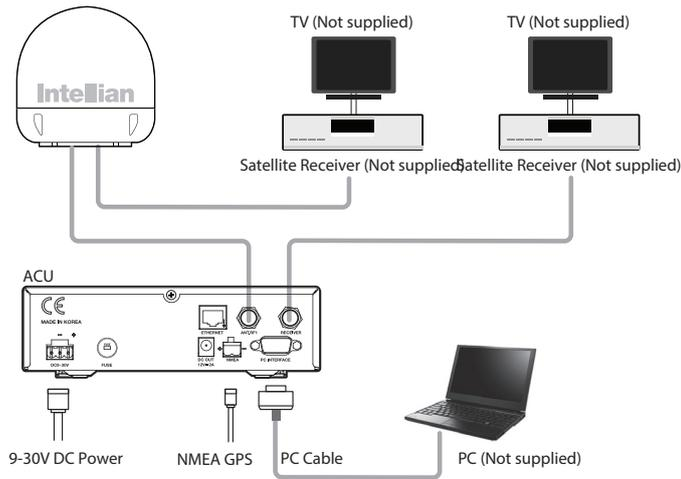
**Figure 01 : Basic System Configuration**
