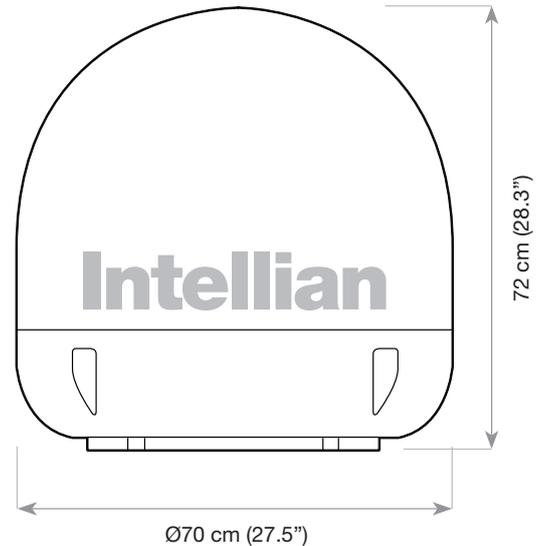
**Figure 08: Radome Dimension of i6/i6P**
