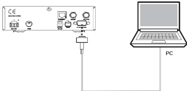
Figure 26 : Serial Connection
