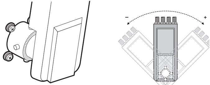
Figure 20 : LNB Skew Angle Adjustment
