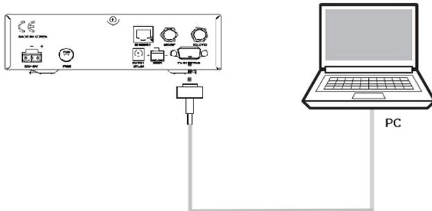
Figure 26 : Serial Connection
