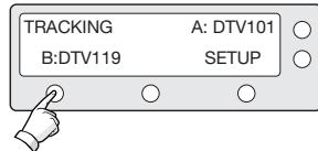
1. Press LEFT soft key for tracking Satellite B.
