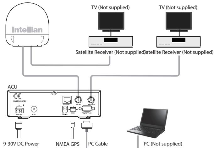
**Figure 01 : Basic System Configuration**
