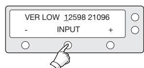
8. Input the tracking frequency (MHz) and symbol rate (KHz) for vertical low band.
