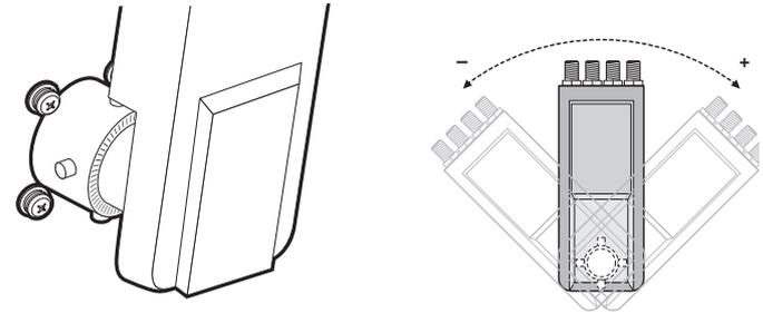
Figure 20 : LNB Skew Angle Adjustment
