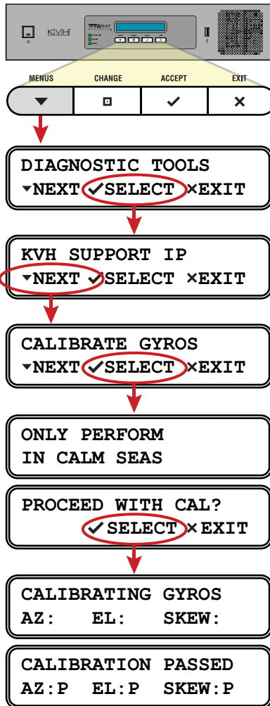
Figure 9-13 Calibrating the Gyros
