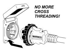
To use the Easy Lock System, align the lock locator tabs on the Easy Lock ring on the cordset with the slots on the sides of the threaded boss on the inlet. Push the Easy Lock ring onto the boss and twist 1/8 turn for a positive water-proof connection.
