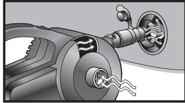
2. Attach adapter nozzle to inflation end of pump. Insert pump and turn on.
