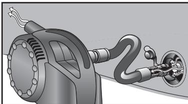
Remove adapter hose from inflation end and attach to opposite deflation end of pump. Repeat same steps as inflation. This will draw the air out quickly.
