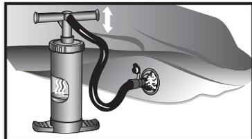
2. Attach adapter nozzle to inflation end of pump. Insert pump and turn on or start pumping.
