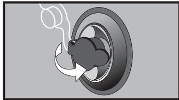
4. Fully remove pump and close external cap. Valve should appear depressed into itself.
