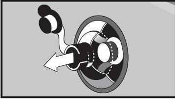
1. To begin inflation, open external cap and pull firmly on the lanyard to extend out. This will open internal yellow seal.
