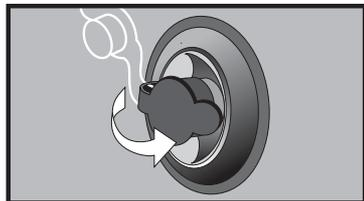
4. Fully remove adapter and close external stopper. Valve should appear depressed into itself.
