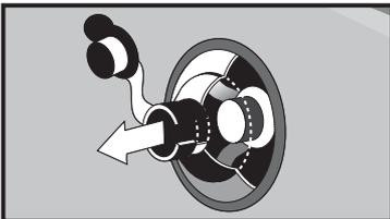
1. To begin inflation, open external cap and pull firmly on the lanyard to extend out. This will open internal yellow seal.
