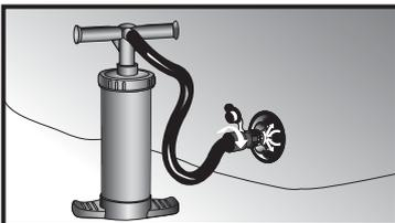
3. When fully inflated, seal valve by pushing in with pump nozzle. This will seal the internal yellow stopper and keep air from escaping while closing cap. Gently twist adapter sleeve to right while backing pump out of valve.
