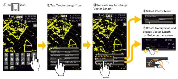
Sets TT and AIS vectors. The bearing and speed signal input are required to display TT and AIS vectors.
