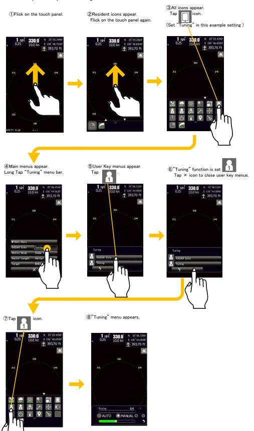
It is possible that you can give your favorite function to the option key . By using the option key, you can open the heavily used menu in one operation. You can set a function listed in the "bar menu" to an option key as following. However, the functions performed by an icon cannot assign to the option key.
