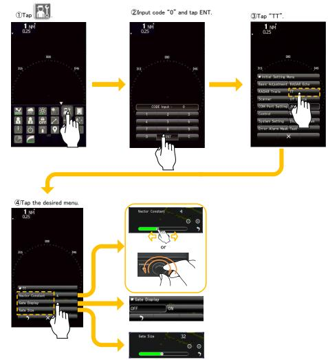
Vector Constant: Vector shows the movement of the target. When Vector Constant is large, vector is stable, but the response is slow. When Vector Constant is small, vector is unstable, but the response is quick.
