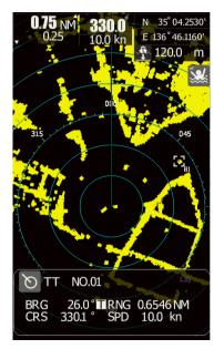
When selecting a tracking target to display its numeric information, this symbol is superimpose-displayed on the selected target. This is displayed with a split square (basic color is white). This is superimpose-displayed on tracking targets, new tracking targets or dangerous targets. Assigned the ID number automatically.
