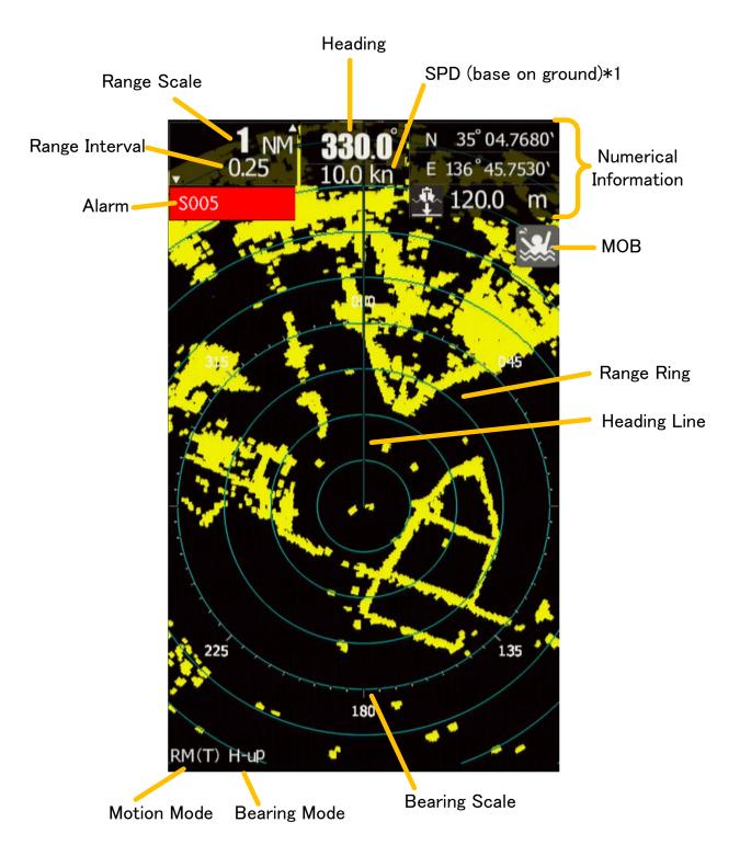
$\ast 1:$  In case of only input of VHW, it indicates speed through the water
