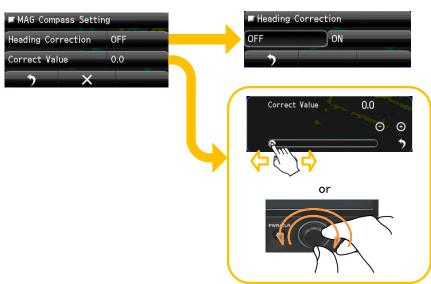
This item is set as to whether or not the heading bearing is to be corrected. Switches between On and Off.
