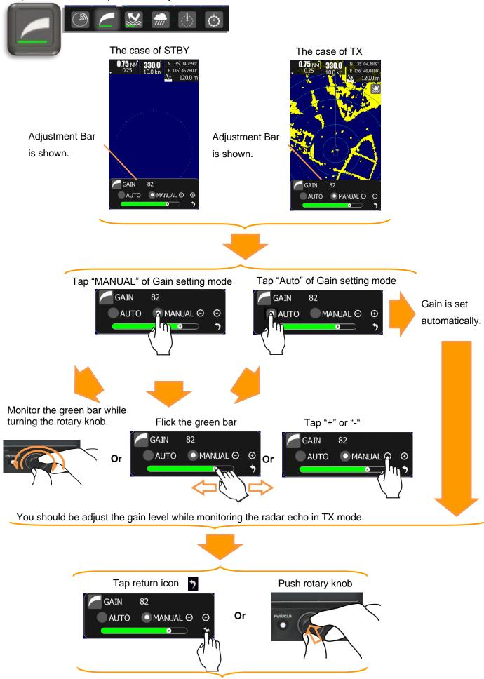
Push the rotary knob or tap the return icon to fix the setting.
