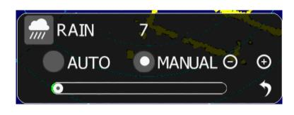
How to change the RAIN clutter suppression level: Please refer to the rain clutter suppression adjustment method described in Chapter 2.4.3.
