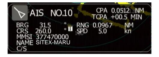
CPA: CLOSET POINT of APPROACH TCPA: TIME to CPA BRG: Target BEARING from own ship direction RNG: Target RANGE from own ship position CRS: The ship's course of ground SPD: The ship's speed of ground MMSI: The ship's MMSI NAME: The ship's name C/S: The ship's CALL SIGN
