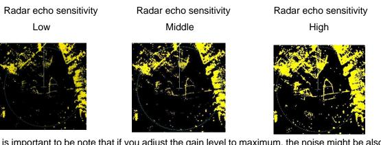
It is important to be note that if you adjust the gain level to maximum, the noise might be also displayed on the screen at the same time.
