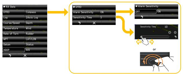
Do not change the set value carelessly. If alarm detection is turned off or detection time is changed, be careful because the alarm may not occur or may be delayed.
