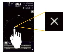
To use the "Symbol marker" function, GPS signal input is necessary because symbol position is memorized as a latitude and longitude data. If no GPS signal is input, you cannot select "Symbol marker" function.
