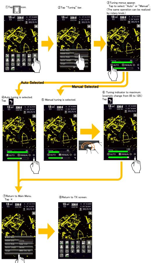
Automatic tuning mode (AUTO) and manual tuning mode (MANUAL) are provide. In the automatic tuning mode, transmission and receiving frequencies are tuned and adjusted automatically. In the manual tuning mode, tuing is carried out by yourself.
