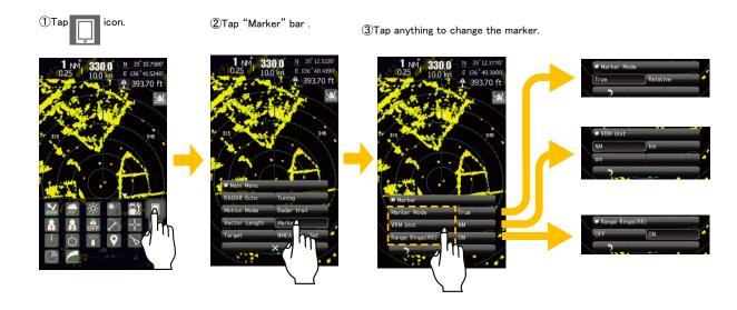
Marker Mode sets whether to display EBLs in true bearing mode or relative bearing mode. Bearing signal input is required to display true mode.
