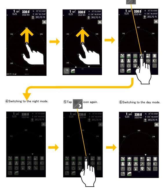
Combination of the display color and brilliance according to the ambient lighting conditions is provided. The display color setting can be changed easily.
