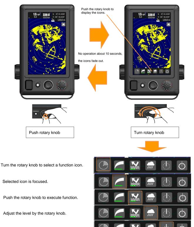
Push the rotary knob to fix the setting. (The same adjustment can be realized by a touch operation.) Tap the TX/STBY icon, or push the rotary knob when the TX/STBY icon is focused.
