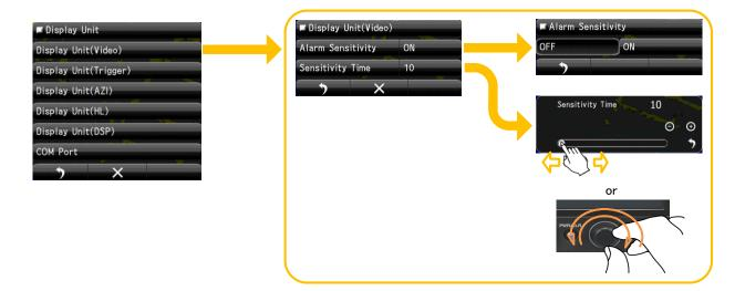
Do not change the set value carelessly. If alarm detection is turned off or detection time is changed, be careful because the alarm may not occur or may be delayed.
