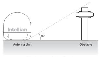
Figure 07: Elevation Limit of Obstacles
