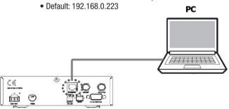
Figure 28 : ACU to PC TCP/IP Connection
