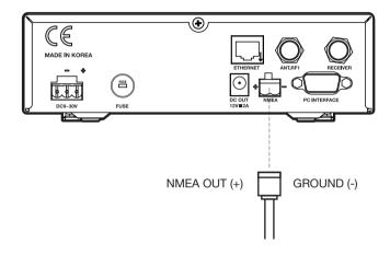
Figure 19: NMEA 0183 GPS Connection
