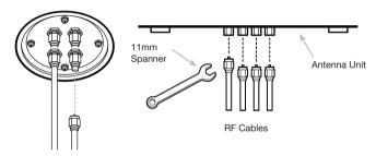
Figure 12: Connectors on Bottom of Antenna
