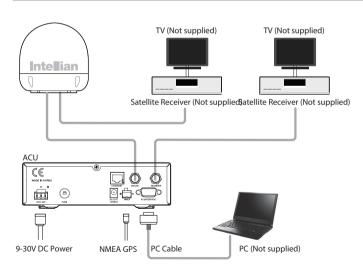
Figure 01: Basic System Configuration
