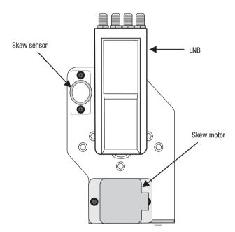
Figure 21: Auto LNB Skew Angle Adjustment
