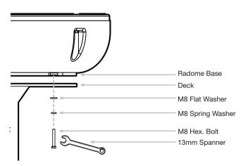
Figure 13: Mounting the Antenna
