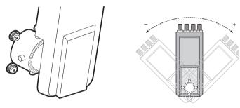
Figure 20 : LNB Skew Angle Adjustment
