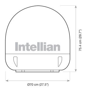
Figure 09: Radome Dimension of i6PE
