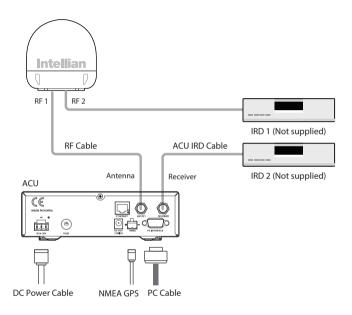
**Figure 17: Dual Receiver Connection**
