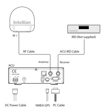
Figure 16: Single Receiver Connection
