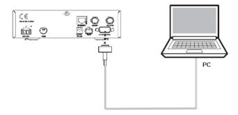
Figure 26: Serial Connection
