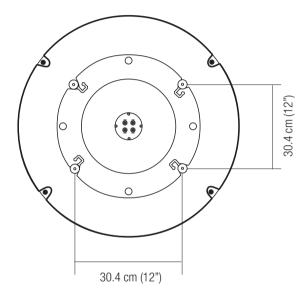
Figure 10 : Mounting Hole Position of I6/I6P/I6PE
