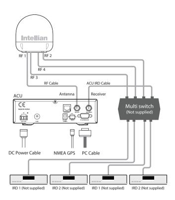
Figure 18: Multi Receiver Connection
