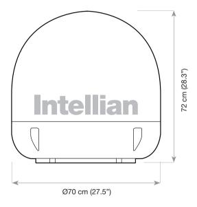
Figure 08: Radome Dimension of i6/i6P
