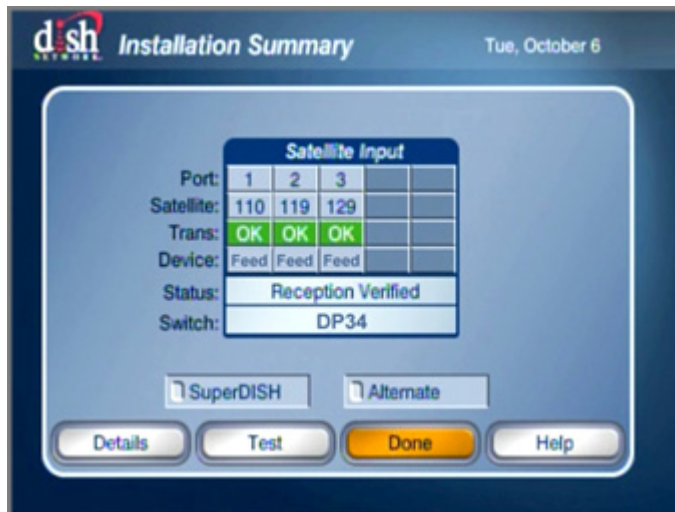
Figure 5-7 Check Switch Test Results
