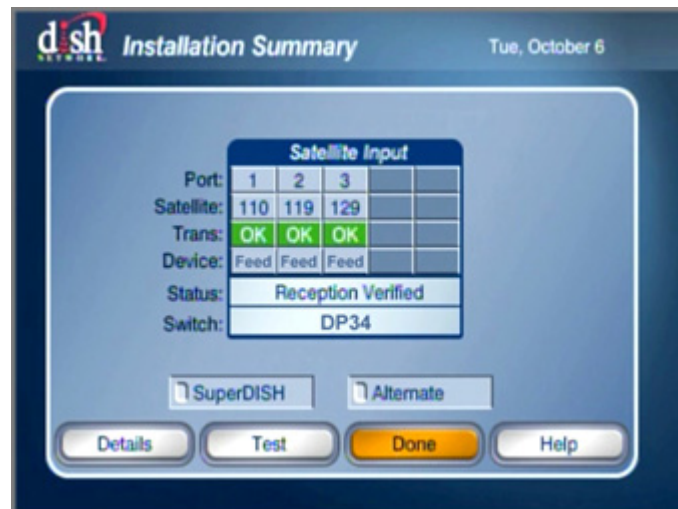
Figure 5-8 Check Switch Test Results
