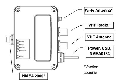
Figure 3 Smartfind M15 Connection Interface
