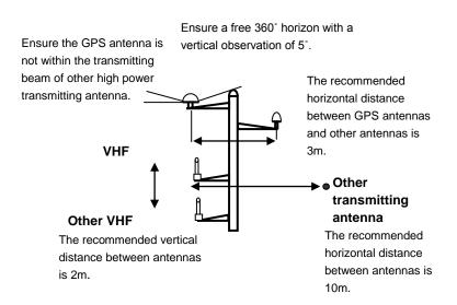
Figure 10 VHF Antenna Installation
