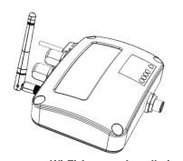
Figure 11 Wi-Fi Antenna Installation
