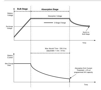
Figure 36 Two-Stage Charging Cycle
