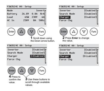
Figure 22 Selecting and Changing a Configurable Setting
