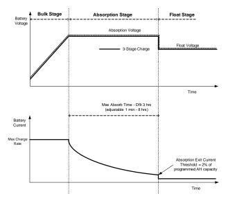
Figure 35 Three-Stage Battery Charging Cycle
