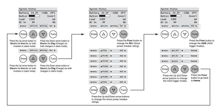
Figure 15 Freedom SW 230V System Status Screen - Soft Key Navigation
