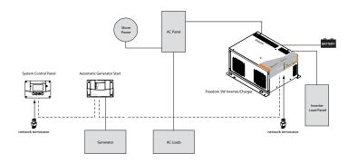
Figure 2 Typical Xanbus System Diagram
