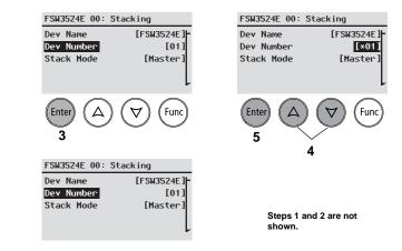
Figure 34 Setting a Device Number
