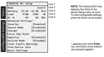
Figure 21 Freedom SW 230V Device Setup Menu
