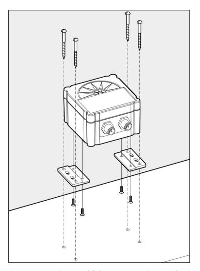
Figure 1 – Mounting the SSC300 to a Horizontal Surface
