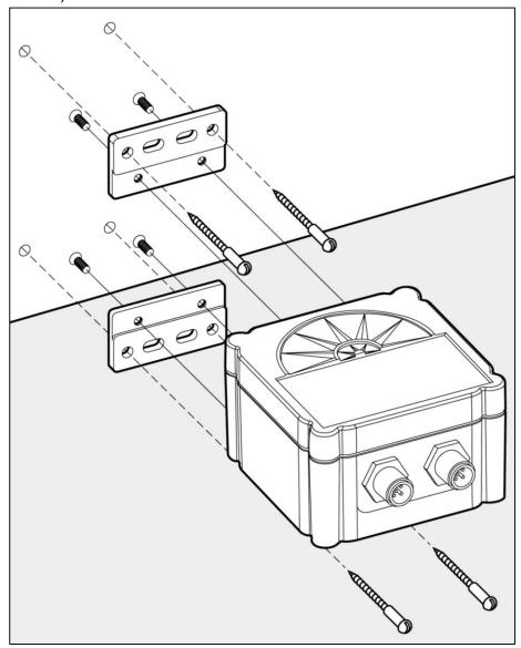
Figure 2 - Mounting the SSC300 to Vertical Surface
