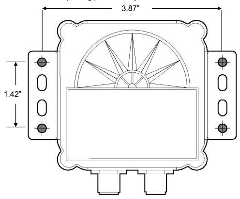
Figure 10 – Horizontal Mounting Surface Template
