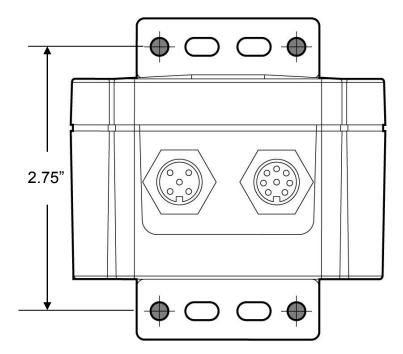
Figure 11 - Vertical Mounting Surface Template
