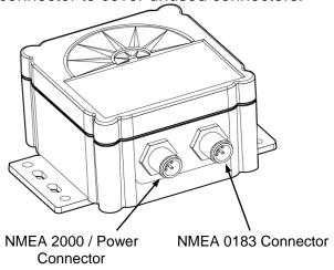
Figure 3 – NMEA 2000® / NMEA 0183 Interface Connector Locations
