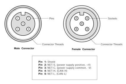
Figure 4 – NMEA 2000®/Power Connector Face Views
