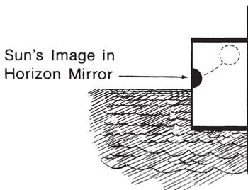
Being careful not to disturb the setting, read the sun's altitude from the scales on the sextant. Since all calculations in the Navigation Tables use the center of the sun or moon, this lower limb reading must be adjusted for semi-diameter correction, shown later.
