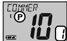
3. To exit from the Preset channel mode, press the [PRESET] key. The trans-
