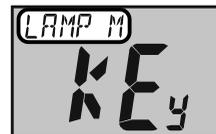
**KEY:** Illuminates the LCD/Keypad for 5 seconds when any key is pressed.
