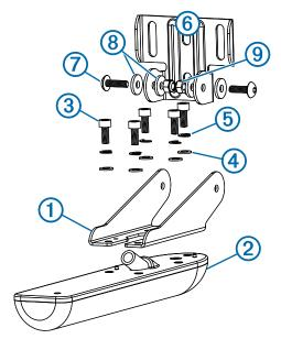
2 Secure the mount to the bracket (6) with the included 12 mm M4 screws (7), M4 flat washers (8), and M4 lock nuts (9).
