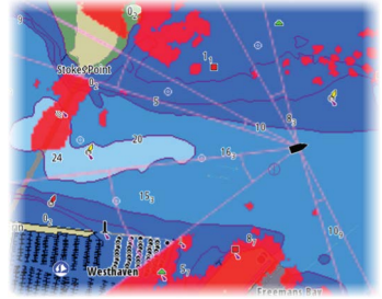
Radar overlay on a chart
