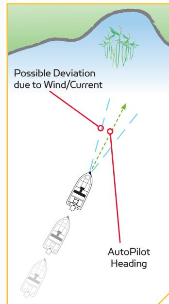
**NOTE:** After steering to a new direction, there is a short delay before the direction is locked in to allow the compass to stabilize. When broad speed changes are made, the AutoPilot heading may change slightly. This is normal.
