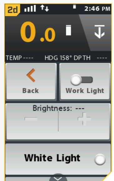
**NOTICE:** When the i-Pilot System is paired with two Talons, toggling the Work Light on the i-Pilot Link Remote for one Talon will toggle the Work Light for both Talons.
