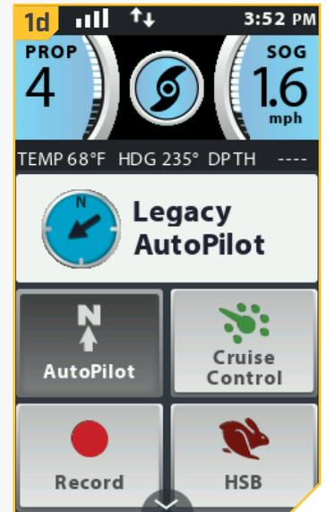
**NOTICE:** If the Prop is not turning or is flashing, be sure to press the Prop Button to enable it. The Prop behavior for AutoPilot can be changed with the Prop Auto On setting. Read "To Toggle the Prop Auto On" section of this manual for more information.
