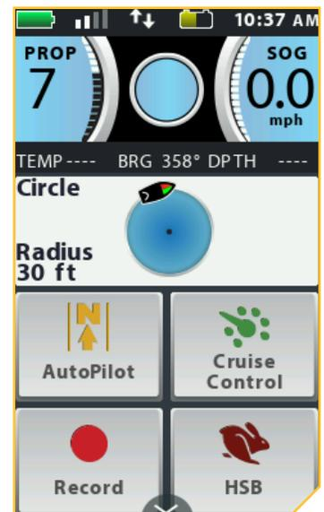
The Circle Mode Active band appears when the navigation is set to Circle Mode. The current circle radius is set to 30 feet.
