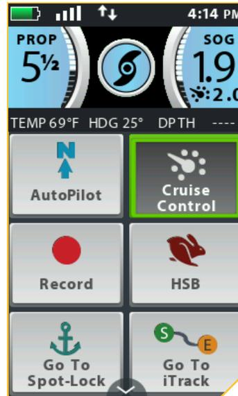
The Home Screen Buttons are Active and the Cruise Control button has been selected using the Screen Navigation
