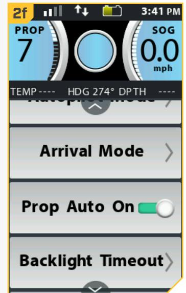
**NOTICE:** Prop Auto On does not affect the Prop when Cruise Control is being used, or when High Speed Bypass is engaged. If Prop Auto On is not working as expected, check the motor speed. The propeller will turn at the current speed setting when Prop Auto On is engaged. If the Prop Auto on feature turns the prop on, and the propeller is not turning, the speed may be set to 0.
