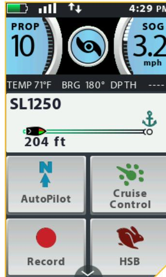
The Go To Spot-Lock Active Band appears when the boat is navigating to a saved Spot-Lock. The Spot-Lock being navigated to is 204 feet away.
