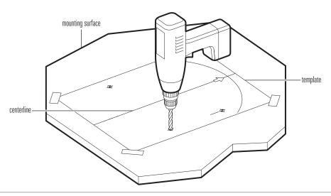
8. **Test the hardware**: Check that each bolt (with spring washer and flat washer) protrudes through the mounting surface at least 5/8" (16 mm) but less than 7/8" (22 mm).
