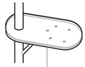
Do not mount on a surface with an edge that might trap water.
