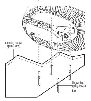
6. Hand-tighten the bolts to a torque of 11 ft-lbf (15 Nm).
