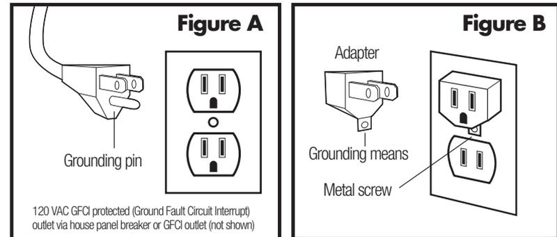
Use of an adapter is not allowed in Canada. If a grounding type receptacle is not available, do not use this appliance until the proper GFCI protected outlet is installed by a qualified electrician.
