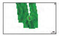
A green circle indicates good depth and GPS position, and a speed under 16 km/h (10 mph). A yellow circle indicates good depth and GPS position, and a speed between 16 and 32 km/h
