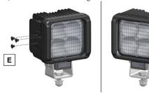
4) Fully Assembled Unit - Drill 7/16" hole in mounting surface for bracket mounting bolt. May be installed upright or inverted
