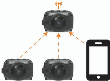
You can also set up a camera network using an existing Wi-Fi network. The app and all cameras connect to the Wi-Fi network. This option is useful when you want to provide internet access to your mobile device while controlling your cameras.
