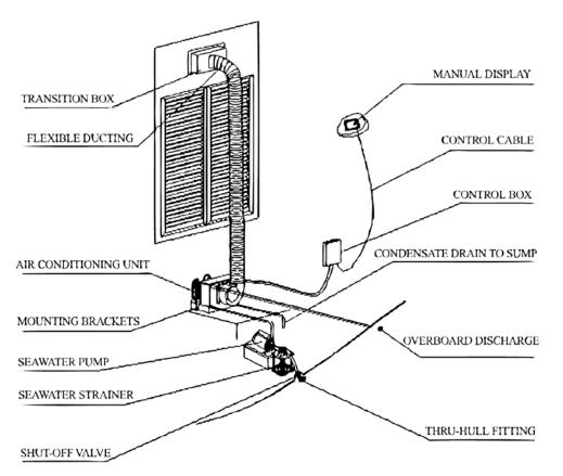
The unit should be installed as low as possible, BUT NEVER IN THE BILGE OR ENGINE ROOM AREAS, ENSURE THAT THE SELECTED LOCATION IS SEALED FROM DIRECT ACCESS TO BILGE AND/OR ENGINE ROOM VAPORS. Installing the unit as low as possible (such as under a V-berth, dinette seat or bottom of a locker) and ducting the supply air as high as possible, creates an ideal airflow condition. This type of installation will prevent short or premature cycling.
