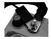
Fig 2.5(a) Temperature Sensor Model EVO-BCTS
