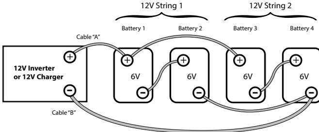
**Fig. 3.7 Series-Parallel Connection**
