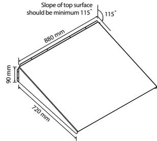
Fig. 3.1(a) Dimensions of Drip Shield
