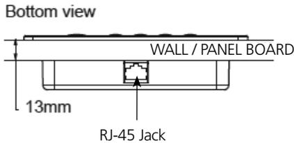
The thickness of the wall/panel board at the place of mounting should not be more than 13mm to ensure that the RJ-45 jack opening is not obstructed.
