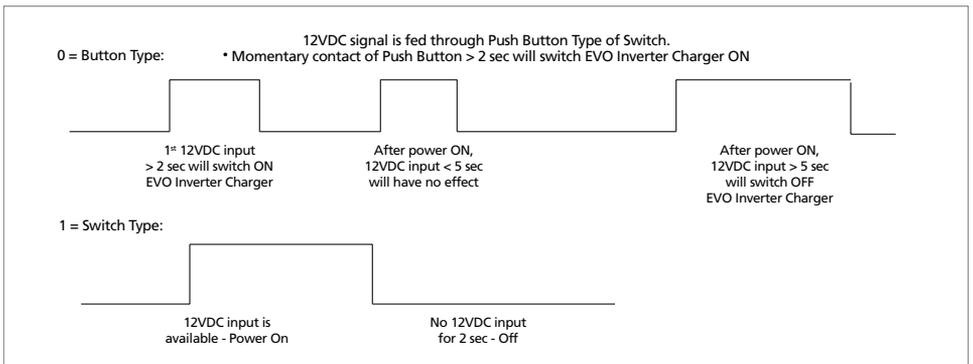
**Fig 4.8. On/Off Logic Diagram for Remote Switch Options**
