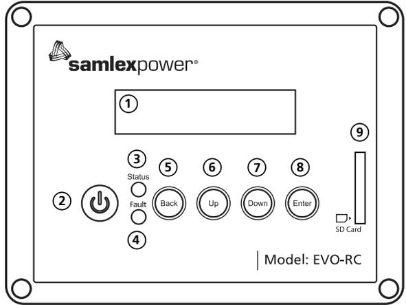
**Fig. 1.1(a) Optional Remote Control EVO-RC – Layout**
