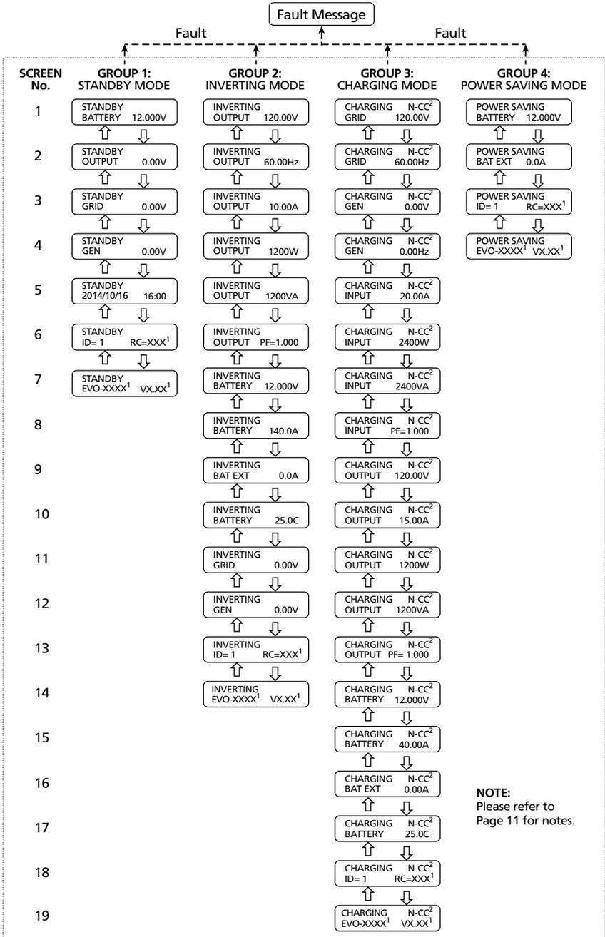
Fig 3.2 Overall Operating Mode Display Screen Menu Map
