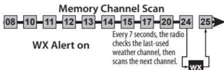
1. If the radio receives a weather alert while scanning, it beeps to alert you that there is an alert on a weather channel. Press any key to stop the alert.
