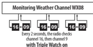
With Dual Watch activated (**MENU/RADIO SETUP/Dual/Tri Watch** menu) while in Weather mode, the radio checks the priority channel, the current marine channel, and then the most recently used weather channel.
