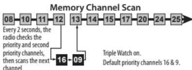
Press **MENU/RADIO SETUP/Dual/Tri Watch** menu or **TRI** soft key again to cancel Triple Watch mode.
