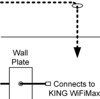
If there was a prewire enclosure on the roof, you will find a preinstalled wall plate in the vehicle. Remove this wall plate and install the included black or white wall plate.
