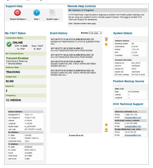
The "My VSAT Status" provides the same basic status information as the Home page, with the addition of antenna pointing information: Azimuth (Az), Elevation (El), and Skew. More detailed status information is provided at the bottom of the page.
