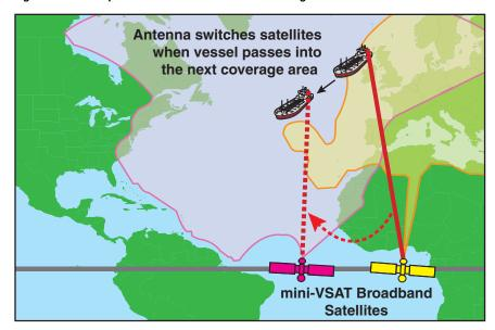
Figure 1-7 Example of Automatic Satellite Switching
