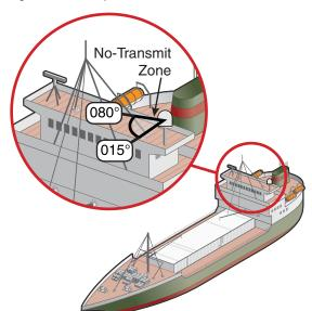
Figure 4-1 Example of a No-Transmit Zone
