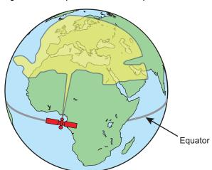
Figure 1-5 Example of a Satellite Footprint
