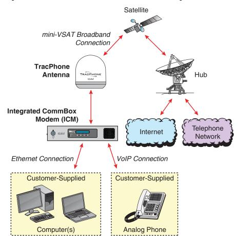
Figure 1-2 TracPhone V3-HTS mini-VSAT Broadband Network Diagram
