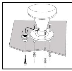
For deck mounting allow the cable to exit the side of the antenna mount and pass through the deck using a suitable deck gland.
