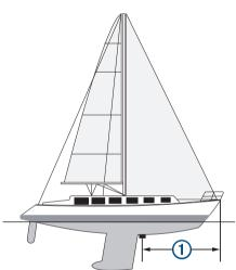
2 From an applicable sonar view, select MENU > Sonar Setup > Installation > Bow Offset.
