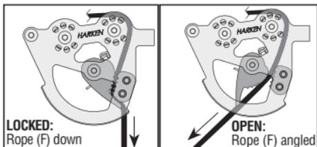
**DIAGRAM 1.** Locked (left): Single black/red hoisting rope (F) pointed straight down locks cleat. Open (right): Angled rope opens cleat.
