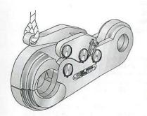
**Sea Catch TR15LM** This is a modified TR15 provided with a front jaw enlarged to receive up to 3.4" fibre line. Additional side plates at the jaw area help spread the load and prevent line chafing. Other capacities are available.
