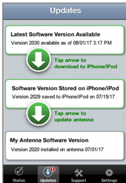
Figure 10-4 Updating Software Using the iPhone/iPod touch App
