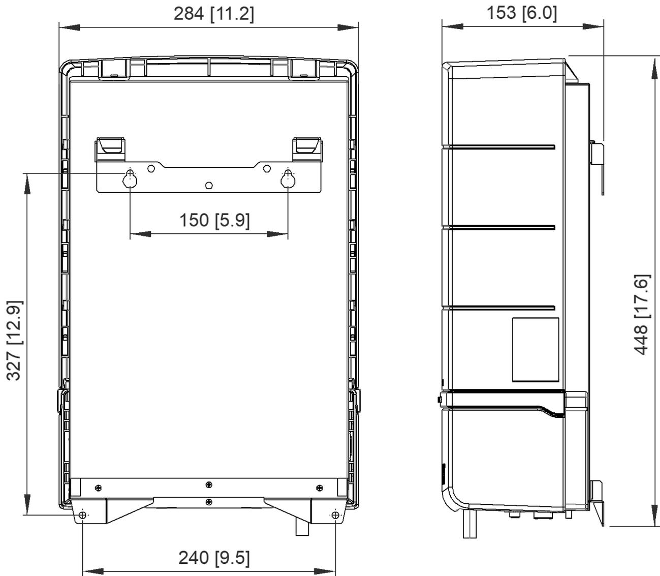
Figure 8: Dimensions 12V/3000VA-100A and 24V/3000VA-60A in mm [inches]
