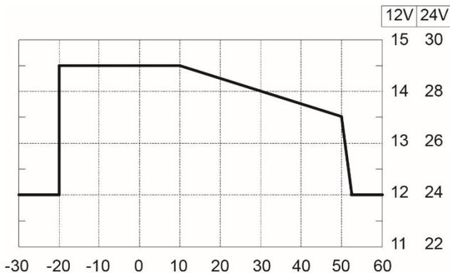
By installing the battery temperature sensor (for Lead Acid batteries only), the charge voltages are automatically adapted for deviating temperatures.
