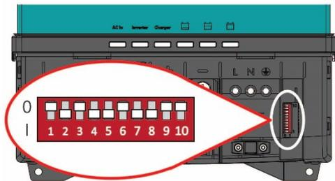
DIP switch 1 = CZone network (0↑) or MasterBus network (1↓).
