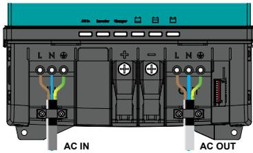
**Step 8.** Integrate a fuse holder in the positive battery wire but do not place the fuse yet! Fit crimp-on cable lugs (M8) to the DC cables. Connect the DC cabling of the battery bank: positive to +, negative to –.
