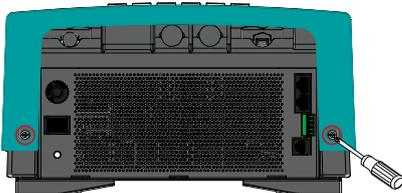
**Step 7.** Connect the AC wiring to the screw terminals. Fasten the cables with a strain relief.
