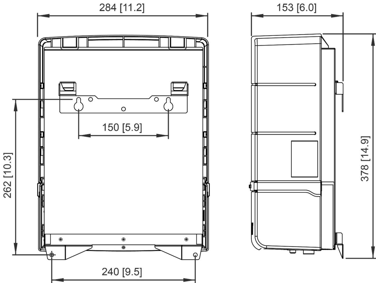
Figure 9: Dimensions 12V/2000VA-60A and 24V/2000VA-40A in mm [inches]
