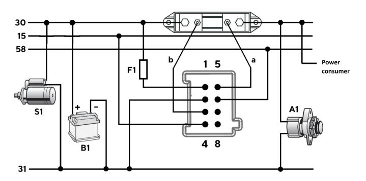
The starter current should not go through the shunt.
