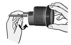
4. Place the bracket on the stud bolt and hand-tighten the knurled nut.
