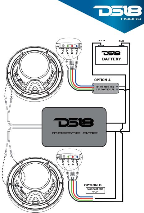
Green Color: "G" Fast Terminal Connect to Battery Negative Red Color: "R" Fast Terminal Connect to Battery Negative Blue Color: "B" Fast Terminal Connect to Battery Negative Purple Color: "R" And "B" Fast Terminal Connect to Battery Negative Yellow Color: "R" And "G" Fast Terminal Connect to Battery Negative Cyan Color: "B" And "G" Fast Terminal Connect to Battery Negative While Color: "R" And "B" And "G" Fast Terminal Connect to Battery Negative
