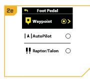
**NOTICE:** Use the Steer Right button to customize the function of the One-Boat Network button. When selected, the radio button next to the desired function fills in. AutoPilot is the default selection for Ulterra QUEST and Riptide Instinct QUEST series trolling motors. The function options listed are specific to the trolling motor and additional devices paired with the Advanced GPS Navigation network.
