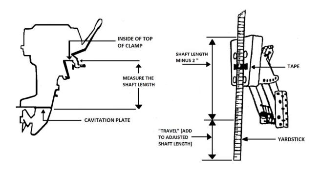
Once you have your measuring stick in place, position the outboard motor bracket on the transom of the boat on either the starboard or port side. Care should be exercised to make sure that the bracket will not interfere with the movement of the existing engine or a rudder.
