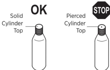
**FIGURE 3** CO<sub>2</sub> CYLINDER CHECK
