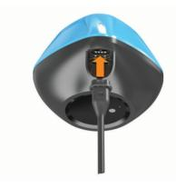
2 Plug the large end of the USB cable into a USB charging port.
