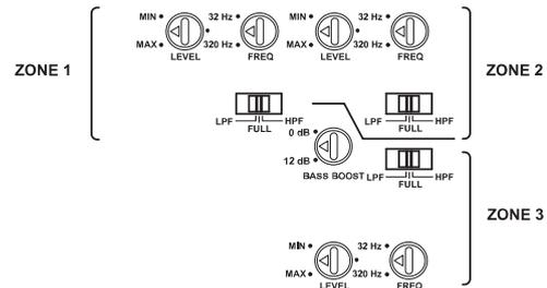
Each zone has a set of controls you must use to configure the sound for the speakers connected to that zone.
