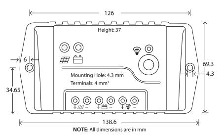
Fig 3.1: Dimensional Drawing of Charge Controller MSK-10A
