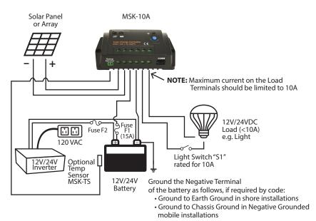
Fig 3.2: Wiring Diagram
