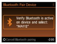
While the unit counts from time -2:00 use your mobile device Bluetooth function to search for a Bluetooth device. The mobile device will display the Bluetooth device name (MA112). Select MA112. Once connected the
