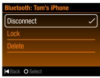
**CONNECT/DISCONNECT:** To disconnect a paired device, press the **VOL/ENTER** button (4) to temporarily remove the Bluetooth connection. The connection can be re-established trough your phone menu by selection the MA112 for connection or select the phone device name on pairing list through the radio unit and press **VOL/ENTER** button (4) select CONNECT for connection.
