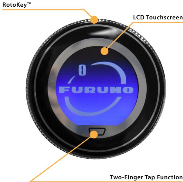
TZtouch2 and TZtouch3 operation is accomplished by utilizing these 3 controls: RotoKey™, LCD Touchscreen, and Two-Finger Tap Button.
