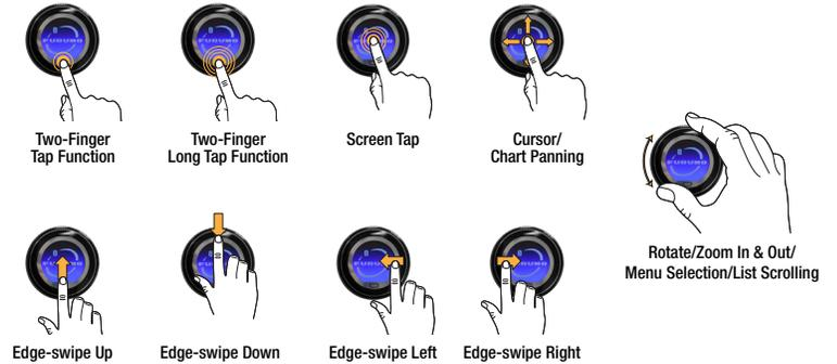
Tips: To automatically close menus faster, set the "User Interface Auto Hide" in the General menu from the default of 10 seconds to 5 seconds, or even 3 seconds. In the General menu, set one of the "Two-Finger Tap Functions" to "Gain Control." This is a quick way to access the manual gain controls of the Fish Finder, DFF3D, and Radar.
