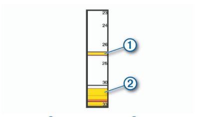
The a-scope above shows fish returns  $\bigcirc$  and a soft bottom return  $\bigcirc$ .
